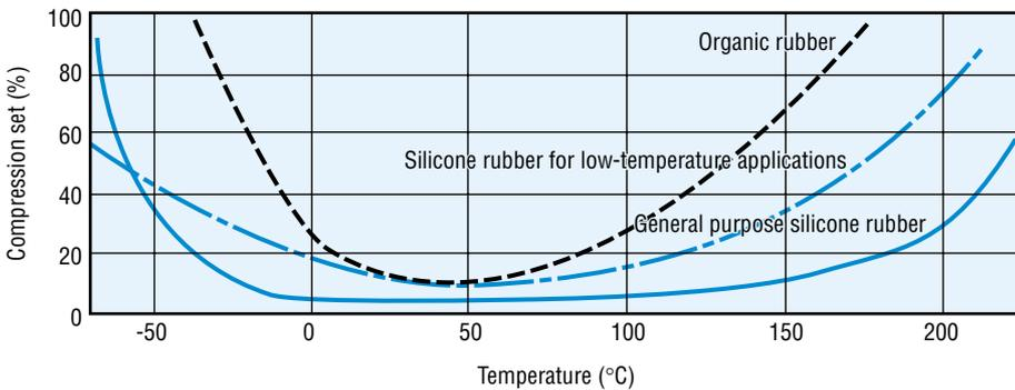
\* Creep is the deformation of a plastic material under constant load. Typically, creep increases as temperature rises. Rubbers that are firm and have greater thermal stability tend to exhibit lower creep values at higher temperatures. Silicone rubber exhibits less creep than organic rubbers, and is more stable even than fluoro-rubber, which has good heat resistance.
