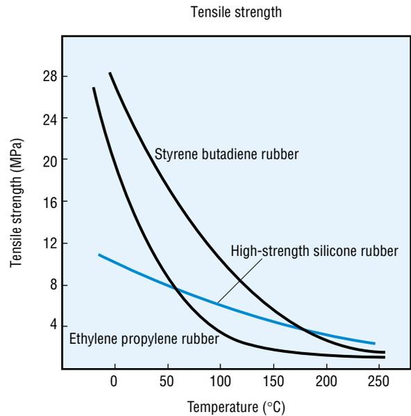
\* The strength of silicone rubber at room temperature is inferior to that of organic rubber, but silicone rubber maintains strength better at high temperatures, such that the two eventually trade places on the graph.
