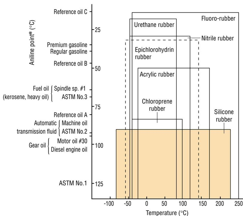
\* Aniline point: the lowest temperature at which equal portions of an oil and aniline are completely miscible. The lower the aniline point, the greater the swelling effect of the oil.
