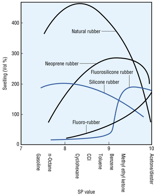
The solvent resistance of fluorosilicone rubber is particularly high, although all silicone rubbers resist solvents better than other types of rubber.
